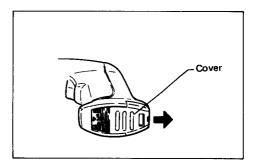
Withdraw the built-in battery halfway. Disconnect the two lead wires from the battery by pulling them from the battery terminals. Then withdraw the battery completely.
